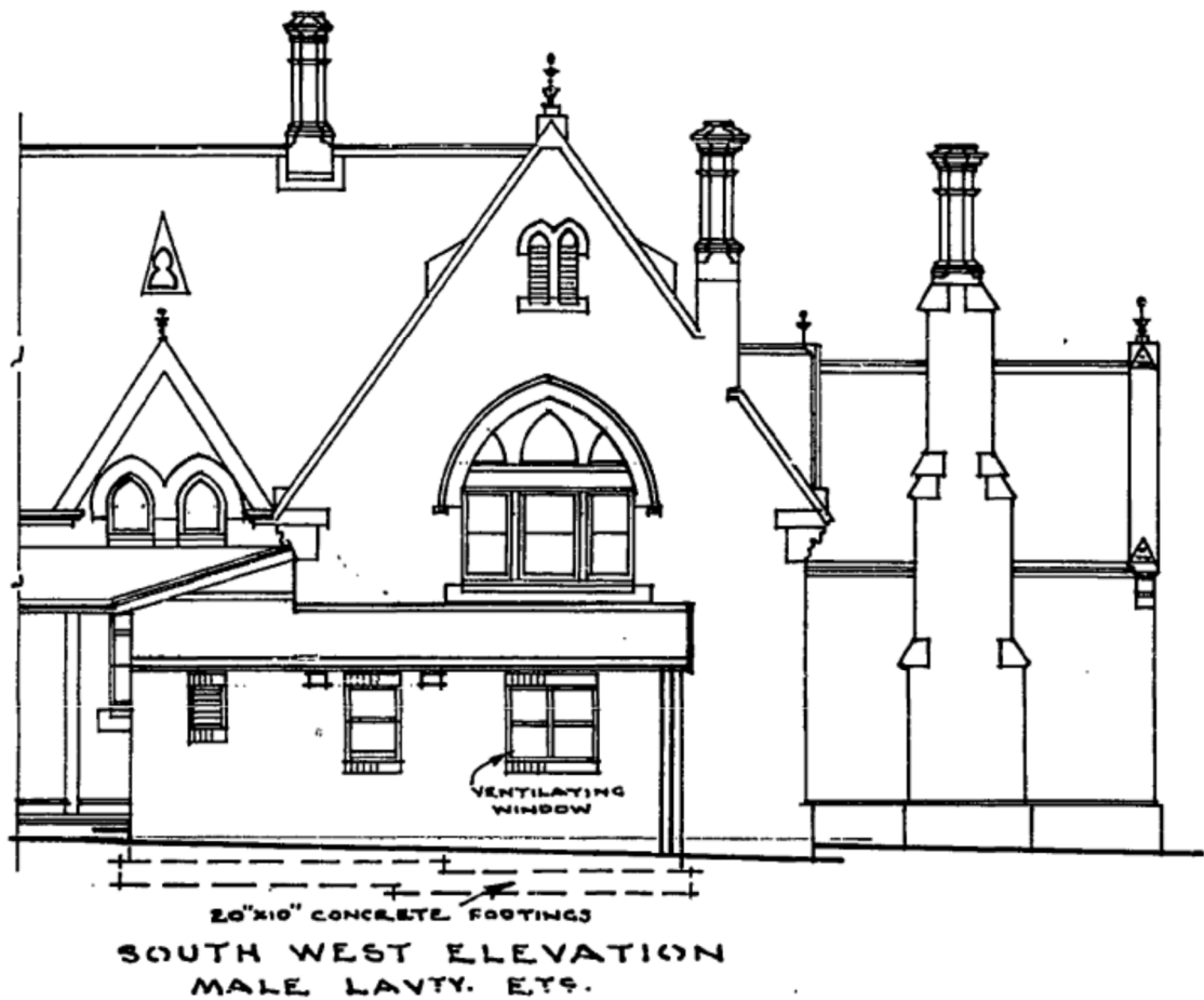
Figure 4 – South-West elevation from 1940 drawings for amenities extension.
